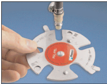
Install on pneumatic fitting
