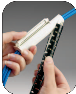
Slide PAN-WRAP Split Harness Wrap onto end of tool until approximately 3 inches of it covers the bundle.
