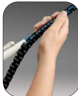
Grasp end of PAN-WRAP Split Harness Wrap and bundle while pulling the tool along the bundle length.
