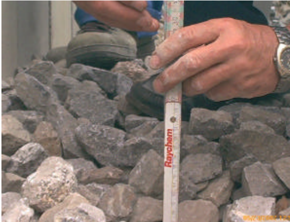
Fig. a: Samples covered by 10cm grit
