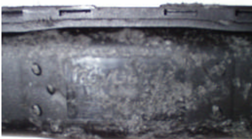
Fig. e: RayGel-24 after the joggle test
